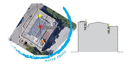
Figure 1. Location of the new and old antenna in plane view (left) and in vertical view (right).
