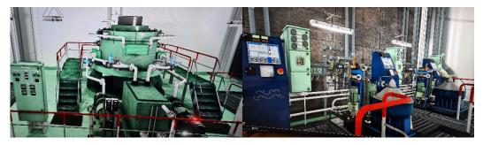
Figure 4. Steering gear and the purifiers in the marine engine room simulator (left to right).
