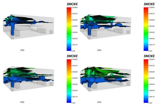
Figure 5. Smoke concentration in 10-minute period after ignition
