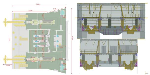
Figure 1. Ship engine room CAD model
