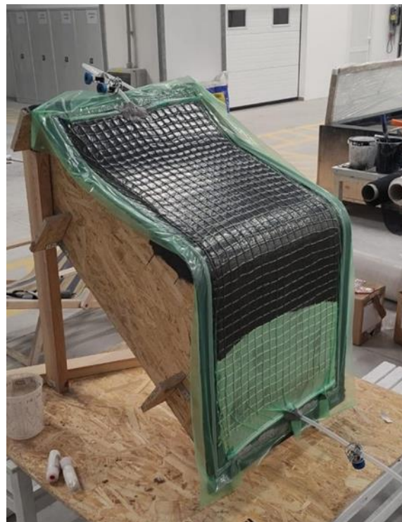
Figure 2. Seat vacuum infusion.
